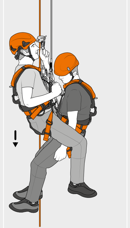
Lowering from an anchor
